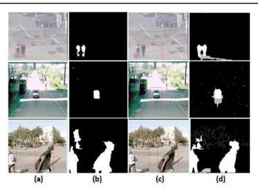
Figure 3. (a) and (b) results for removing the shadow, (c) and (d) tresults for shadow detection
